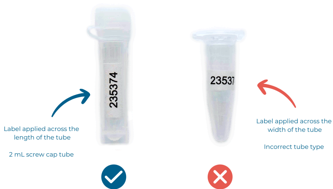
Figure 2. How to correctly apply labels to your tubes. Please use the tubes we provide, or if supplying your own, ensure they are 2 mL thread capped tubes containing 500 \mu L of DNA/RNA Shield Inactivation Buffer .
