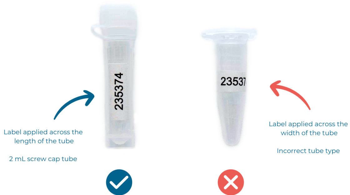
Figure 2. How to correctly apply labels to your tubes. Please use the tubes we provide, or if supplying your own, ensure they are 2 mL thread capped tubes containing 500 \mu L of DNA/RNA Shield Inactivation Buffer .
