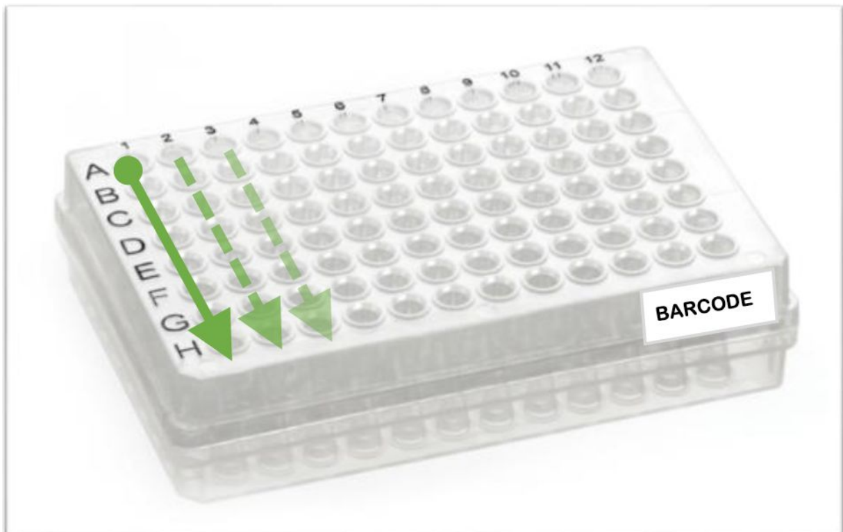
PICTURE 3. HOW TO LOAD SAMPLES IN A 96-WELL PCR PLATE. Load by columns starting in well A1.
